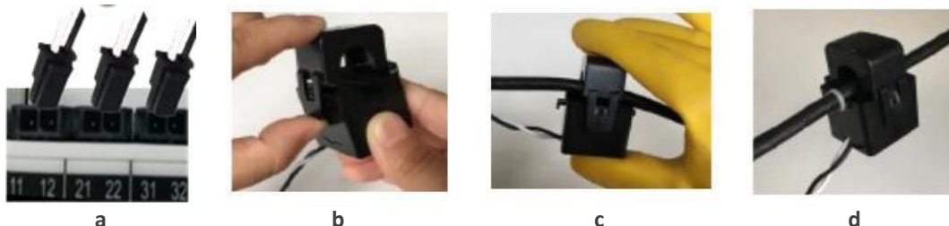
Figure 2-14 5A/2mA, 100A/40mA, 200A/40mA or 400A/40mA SCCT Installation
