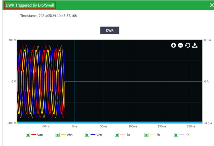
Figure 3-77 SOE Detail about DWR Triggered by Dip/Swell
