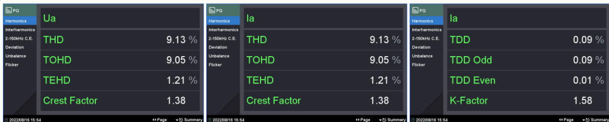
Figure 3-21 Voltage and Current Harmonics Large Font Displays
