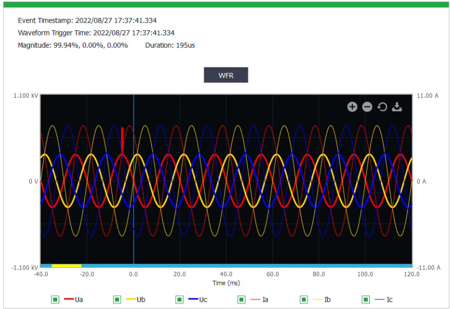
Figure 4-11 Transient Event @ 512 samples/cycle x 100 cycles
