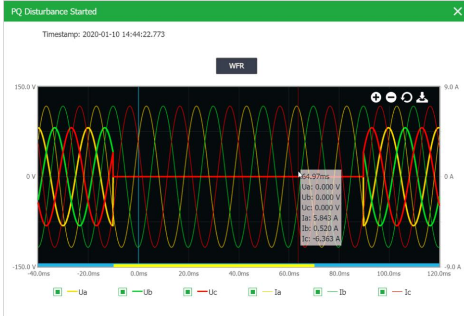
Figure 3-99 PQ Disturbance Started (Interruption triggered by UA)
