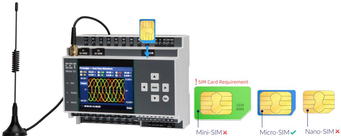
Figure 2-12 SIM Card Installation
