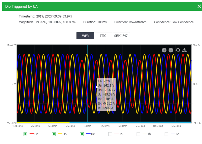
Figure 4-8 Dip Event @ 1024 samples/cycle x 40 cycles
