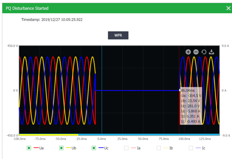
Figure 4-10 Interruption Event @ 1024 samples/cycle x 40 cycles
