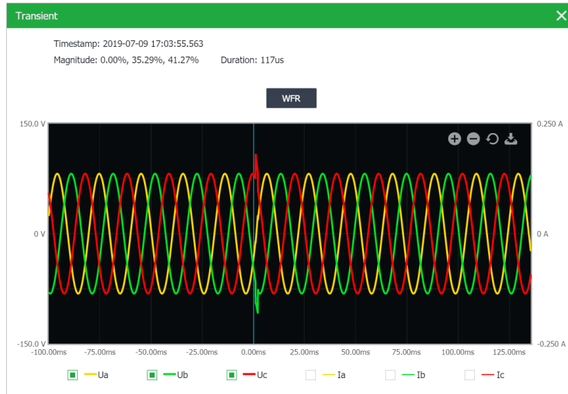
Figure 4-11 Transient Event @ 1024 samples/cycle
