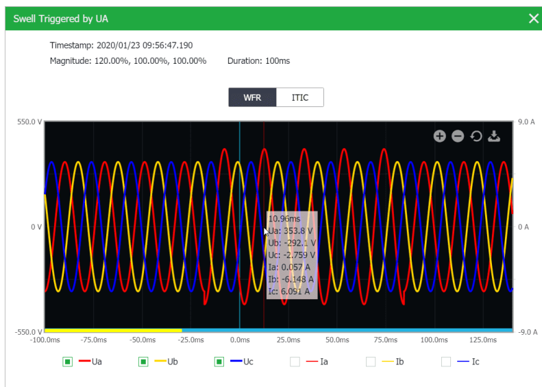
Figure 4-9 Swell Event @ 1024 samples/cycle x 40 cycles
