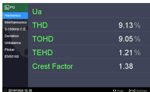
Figure 3-23 Large Font Display for Harmonic Measurement
