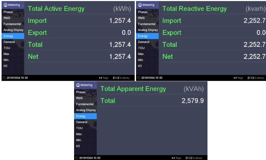
Figure 3-11 Large Font Displays for RMS Energy Measurements
